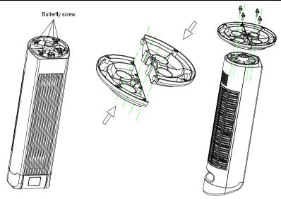
Unpack your heater and remove both halves of the base from the package. Refer to the picture below:
